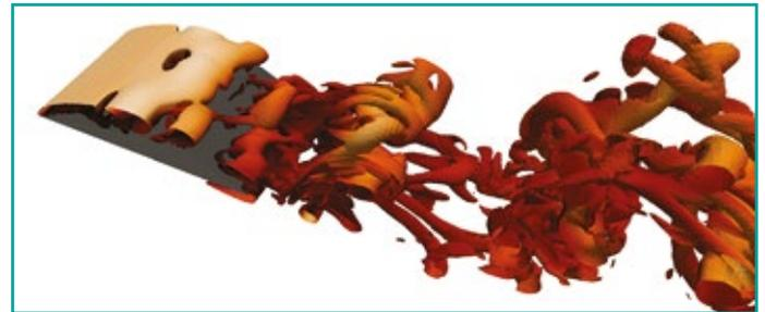
Images from simulations of optimized airfoils showing the vortices being shed off the leading edge and apex of the airfoils that then break down into three-dimensional structures. (Images: L. Caros, O. Buxton and P. Vincent 2023)
