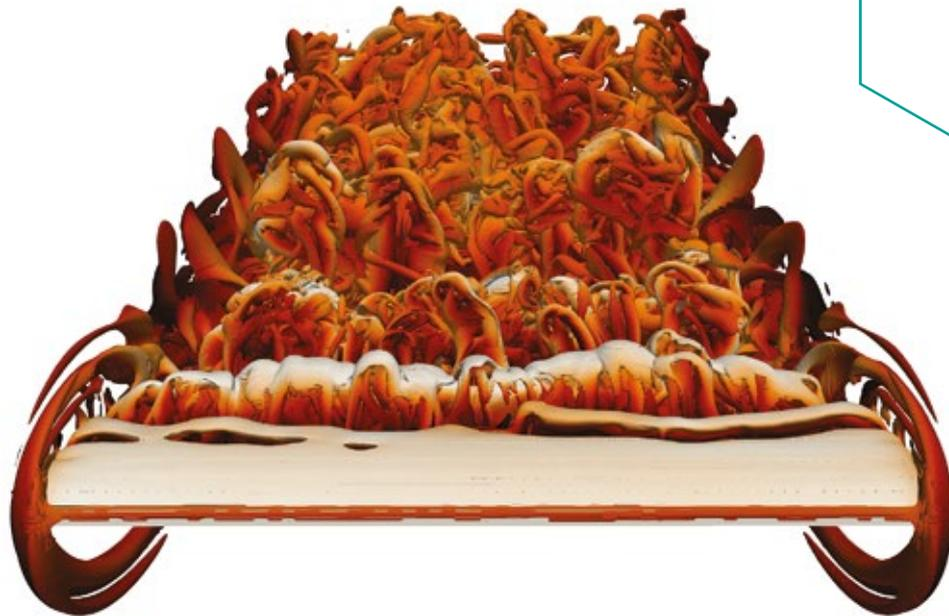
To tackle these issues, researchers at Imperial College have been conducting high-fidelity Computational Fluid Dynamic simulations using the Cirrus supercomputer, focusing on developing airfoil shapes optimized for Martian conditions. Drawing inspiration from the aerodynamics of dragonfly wings, which are effective in low Reynolds number environments, the researchers are investigating unconventional designs such as triangular and corrugated airfoils.
